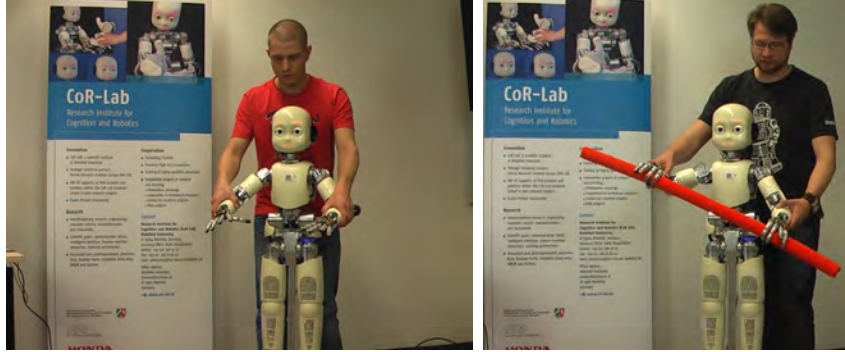
Fig. 12: Experimental setup of the physical human-robot interaction: A human tutor teaches iCub a bi-manual skill without tool [left] and with [right].
