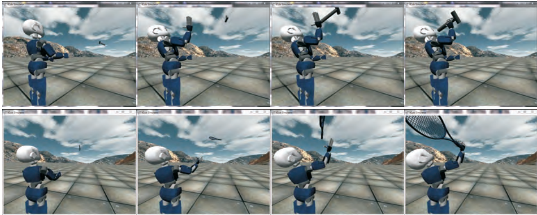
Fig. 8: An hammer and a racket is thrown 3 meter distance from the robot in the iCub simulator. The simulated iCub robot catches the hammer and the racket in the fly.
